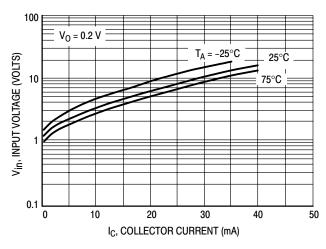
Figure 5. Input Voltage versus Output Current
